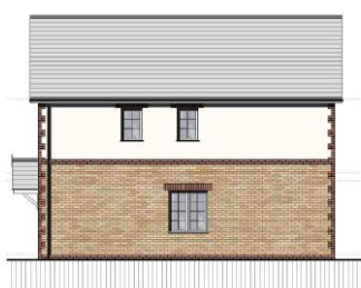
PROPOSED ELEVATION OF HOUSE WITH RENDER BAND (IN LOCATIONS AS IDENTIFIED ON DRAWING PL 110) | 1:100
