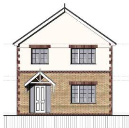
PROPOSED ELEVATION OF HOUSE WITH RENDER BAND (IN LOCATIONS AS IDENTIFIED ON DRAWING PL 110) | 1:100
